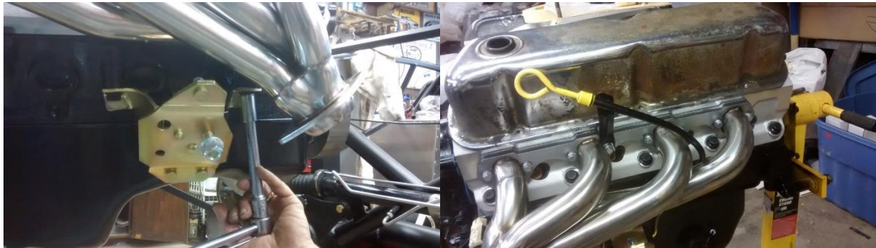
Installing the engine and headers and guess what some things don't go where they are supposed to like the dipstick tube that needed rerouted.
