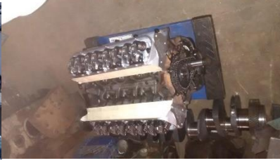
Installing the horns and the day arrived!! Getting the engine home! It's a rebuilt 302 stroked to 347 c.i. for 360 hp.
