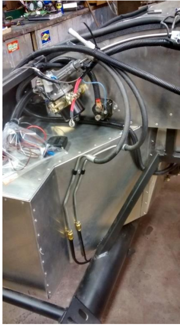
Fuel lines are run and working on the manifold
